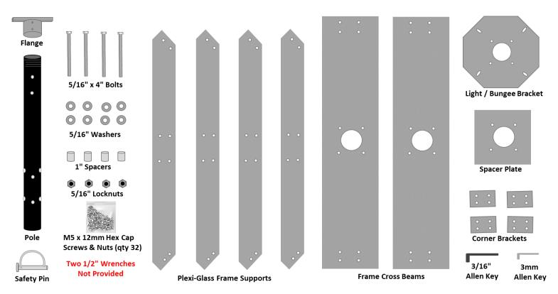
I have found it helpful to use the Megatron's Base and Pole when assembling the Frame. The following step by step pictures show the base and pole being used. Please complete each assembly step as described & shown.
