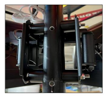
Grab your four TV mounts and the Quad Mount Pole Hardware consisting of a 4 long bolts, 8 washers, 8 saddle spacers, and 4 nuts. You're going to attach two mounts to the pole using 2 bolts, 4 washers, 4 saddle spacers and 2 nuts. Then repeat the steps to firmly attach the other two mounts.
