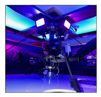
Attach the bungee cords to the top corners of your Light / Bungee Bracket. Make sure you have a helper as you lift up the base up and center the base flange onto the pole. Attach the bungee cords to the corner eye pads of the base and evenly tighten the flange screws to securely level and attach the base onto to the pole.
