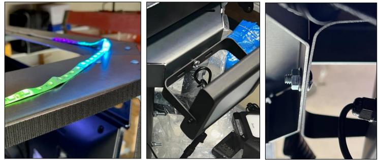
While the frame is in this low position, install the ceiling accent lighting and internal flood lights. The ceiling accent lights can be difficult to shape so just keep it about 2" back from the edge and no one will notice odd bends. Keep the plug near the center of the Jumbotron so the cord does not cast a shadow onto the graphics. Use the four 1/2" screws and nuts provided with your Govee flood lights to mount the flood lights to the Light / Bungee Bracket.
